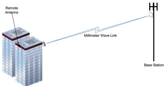
Figure 4: Millimeter Wave Wireless for Distributed Antenna Systems
