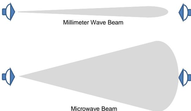
Figure 2: Millimeter wave Links Have Narrow Beams
